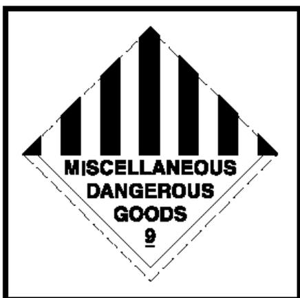
The Class label shall not be less than 250 mm square. It shall be firmly affixed to the vehicle.
